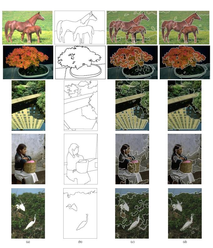
Figure 3. (a) Original image (b) Human benchmark (c) Results of the JSEG method (d) Results of the fractal-dimension-only method.
