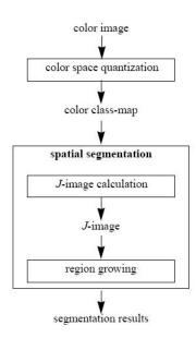
Figure 1. Schematic of the JSEG algorithm [2]
