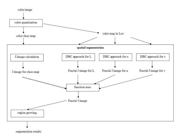
Figure 2. Schematic of the Fractal-JSEG algorithm.
