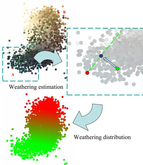
Figure 5. Consider the line segment  $\overline{AB}$ . The weathering degree of a point (green) in the appearance map corresponds to the position of the closest point (blue) in the segment.
