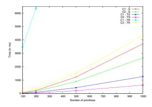
Figure 14: (a) Graph showing times for CC100, CC200, CC500 and CC1000 (each CCx denotes a cylinder subtracted by x cones). Blue line clipped for visualization purposes - its values at 500 and 1000 are 16046 and 34975, respectively
