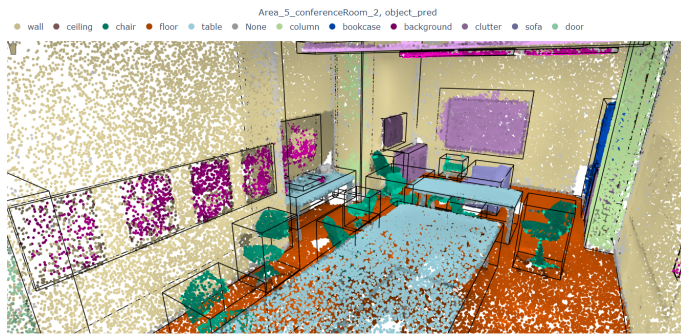
Fig. 4. Object prediction view on Area 5, Conference Room 2 of the S3DIS dataset. Bounding boxes denote approximate predicted object boundaries, and colors denote semantic classification.
