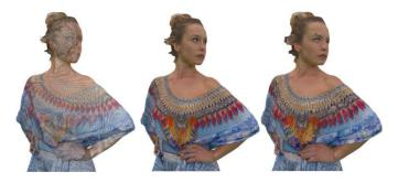
Fig. 2. Voxelization effect for very small (left), proper (middle), and oversized (right) voxel sizes.
