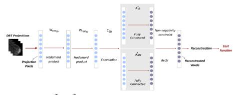
Fig. 1: This architecture can use the layer  $A_{cb}^T$  or  $A_{dbt}^T$  (gray blocks). If the former layer is used, the final architecture represents the Equation 9, proposed by Ref. 3 for CBCT. If the latter layer is used, the final architecture represents the Equation 10, proposed by this work.
