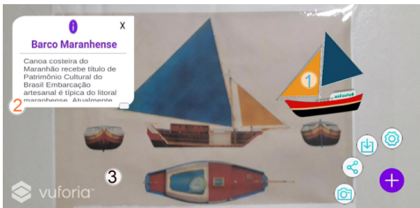
Fig. 5. Image tracked and elements being displayed. In ascending order: 1 - image rendered after object detection; 2 - informative panel containing information based on detected image; 3 - target image.
