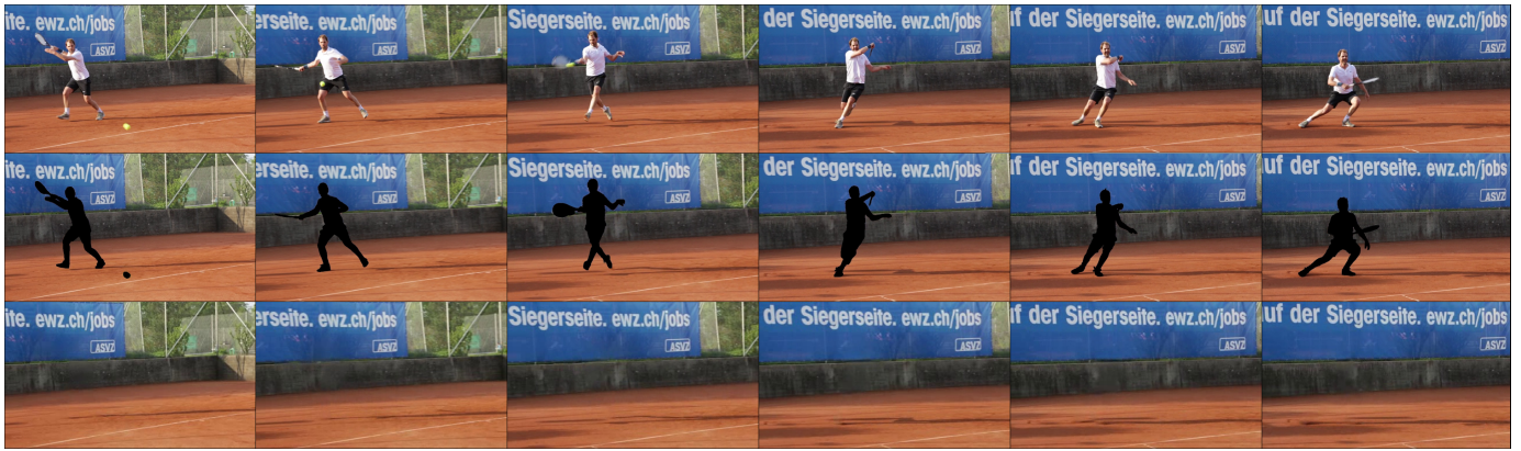
Fig. 1. FastSTTN sample results: our method is capable of inpainting missing regions in video frames efficiently taking into account spatio-temporal information. From the top to the bottom row: original frames, frames with undesirable objects suppressed with segmentation masks, and the resulting inpainted frames.
