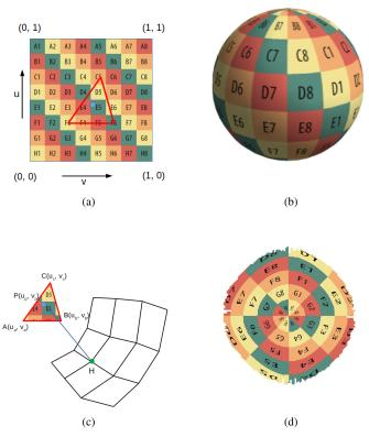
Fig. 4. Reverse texture-mapping process: (a) Texture, (b) The texture applied to the rigid model, (c) Reverse-texture process to obtain texture coordinates for the film mesh from textured rigid model (d) The reversed texture.
