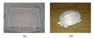
Fig. 1. A 3D printed object covered with carbon fiber pattern by a hydrographic printing technique. (a) Hydrographic film floating. (b) 3D printed object colored with hydrographics.
