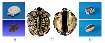
Fig. 10. Color process with two immersions for the turtle model: (a) As input the 3D printed model and the texturized model, (b) the proposed simulation generates the textures to top and bottom. After the physical process with two immersions by using these textures, the turtle is fully colored (c).
