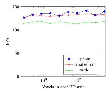
Fig. 7. Variation of FPS by increasing the voxels in each axis of 3D mapped space to collision detection (each value N on x axis corresponds to  $N^3$  voxels). Tests were made with sphere, tetrahedron and turtle models colliding with the film mesh with 21.600 vertices and 42.900 distance constraints.
