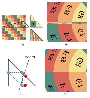
Fig. 5. Some texture coordinates can generate seam problems: (a) triangle with seam problem, (b) seam artifacts are generated, (c) a subdivision scheme is applied by using the midpoint of each edge of the triangle, (d) final result.
