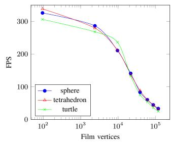
Fig. 6. Variation of FPS by increasing the number of film vertices and constraints (shown in logarithmic scale to x axis) with sphere, tetrahedron and turtle models using uniform grid with  $128^3$  voxels.
