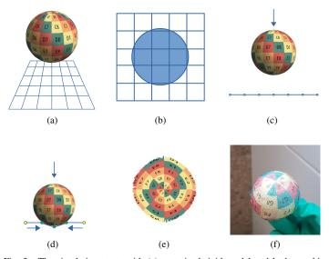
Fig. 3. The simulation starts with (a) texturized rigid model and hydrographic film model. The rigid model (b) is voxelized to collision handling. The simulation moves the rigid body down (c), and handles the collision between the film and the rigid body (d). The texture is transferred to the film with reverse-texture mapping (e). Finally, hydrographic printing is executed in the physical object (f).
