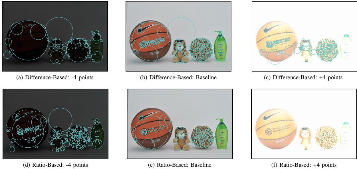
Fig. 7. First scene keypoint detection comparison for N = 128 and extreme exposure configurations. The difference-based approach is displayed in the upper row (a,b and c), while the ratio-based approach is displayed in the lower row (d, e and f). In this example, one can notice how the ability to detect keypoints is reversed when using the proposed approach – the number of detected keypoints is increased for underexposed images, while it is decreased for overexposed ones when compared to the original SIFT approach.
