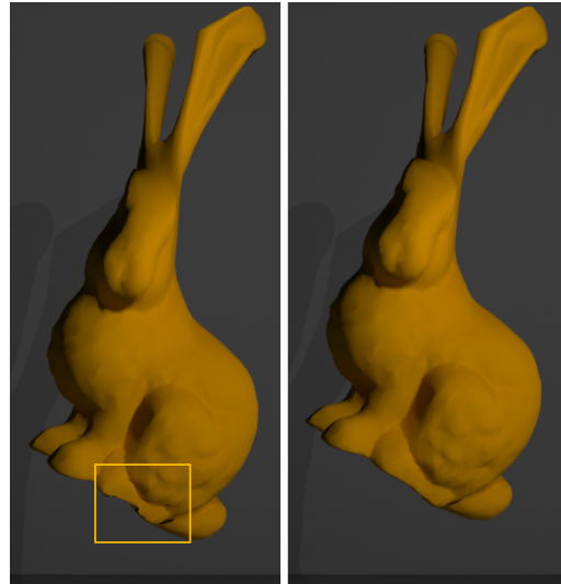
Fig. 5. Bunny model is hanged under constant gravity. St. Venant - Kirchhoff material is simulated. Left: XPBD. Right: Our method. Although both methods behaves identical, our method produces slightly more aesthetic result than XPBD. The difference can be observed on the face and bottom parts of the model.
