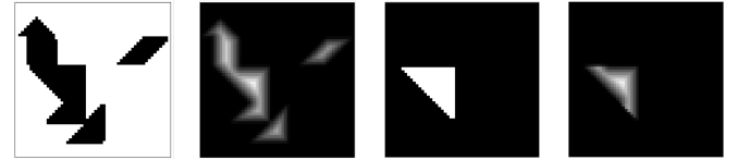
Fig. 9: Process for obtaining the placement cost matrix of the current piece using the distance transform. Pattern mask (left), distance transform (center-left), current piece configuration mask (center-right), and final placement cost matrix (right).
