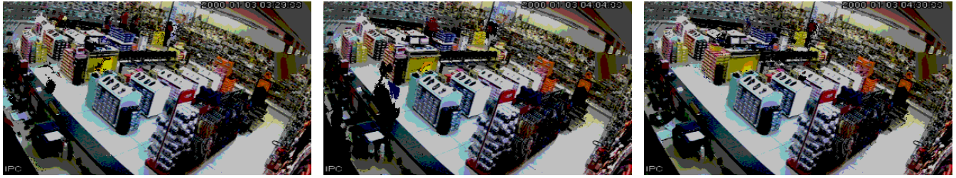
(a) Incorrect background estimation with many salespeople near the entrance (top center). (b) The salespeople gradually begin to disappear with more buffered images. (c) almost correct background with ideal buffer size.
