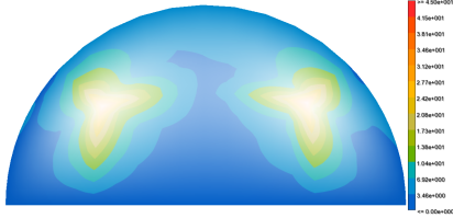
Fig. 19. Alignment quality metric, deviation ( d ) is the color of each vertex and reliability ( \alpha ) the transparency of the color.
