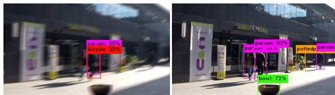
Fig. 1. Object detection using YOLO [5] on the distorted (left) and on the pristine (right) images from GoPro [6] dataset. The detection effectiveness of YOLO is remarkably impaired by the quality of the input image.
