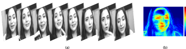
Fig. 2. Using MHI to extract body features. (a) Sequence of frames showing a positive opinion about a book; and (b) MHI representation with an applied jet palette. The lighter gradient values correspond to a greater body movement, darker values represent less body movement.
