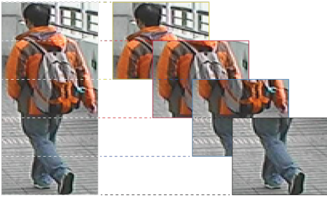
Fig. 2. Illustration of the generated overlapping blocks/chunks. Note that in our approach we generate new samples following a fifty-percent overlap from top to bottom only.
