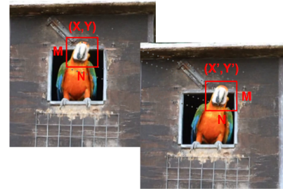
Fig. 4. Example of a macroblock and its respective Motion Vector
