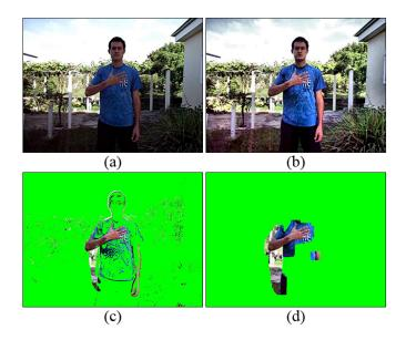
Fig. 3. Results obtained by the pre-processing step: (a) original frame; (b) frame with equalized histogram; (c) frame after applying the background subtraction technique; (d) resulting frame, after applying the closing operation and the median filter.
