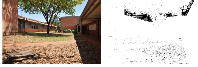
Fig. 5. Overexposed image, captured with 1/800 time exposure (left), and its corresponding saturation map (right).
