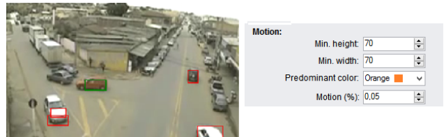
Fig. 2. Search for orange moving objects, 70x70 pixel size minimum.
