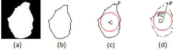
Fig. 2. (a) The hand segmented using the Microsoft Kinect; (b) The hand posture contour; (c) The mass center point drawn in the hand posture contour (dark gray point); (d) The convex hull points with the maximum circumcircle \Theta (red circle), the center mass point (dark gray point), the highest point (red point) and the segment of line \overline{PC} (green line)
