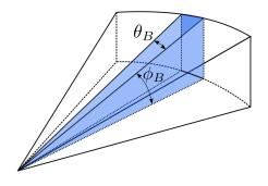
Fig. 2. Single sonar beam's geometry[6]
