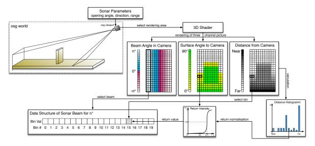
Fig. 1. A graphical representation of the individual steps to get from the OpenSceneGraph scene to a sonar beam data structure.
