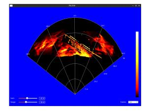
Fig. 5. The simulated forward-looking sonar image.
