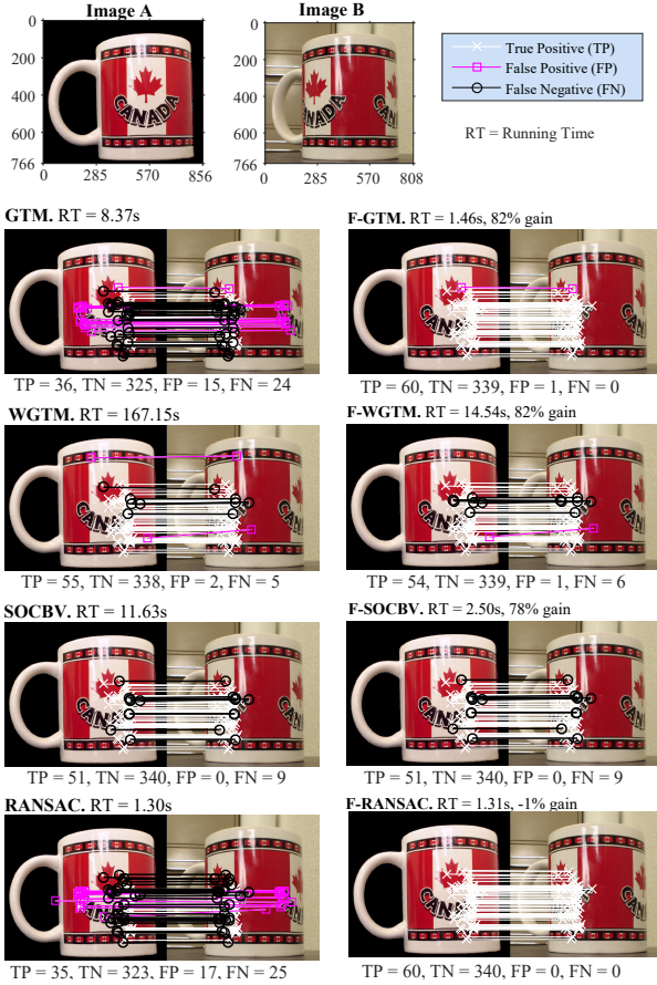
Figure 5. Image matching results for two images from the matching ambiguities dataset (85% of outliers in the initial set of matched points).
