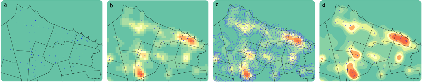
Figure 6. Overview of Marching Square Kernel Density Estimation: in (a) a set of spatial events is selected for the hotspot map. In (b) the KDE hotspot map is generated from the event set. In (c) we see a set of contour lines (in blue) generated after running Marching Squares. In (d) we see the final MSKDE map, after applying an appropriate colormap to regions defined by the contours.
