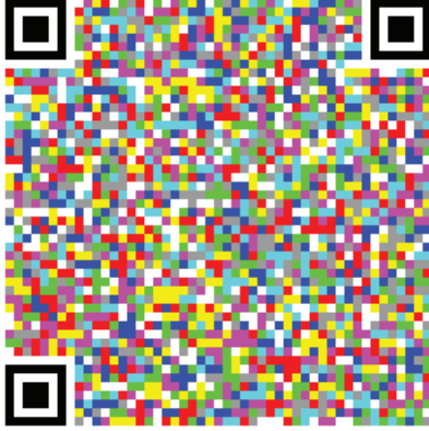
Fig. 8. Example of CQR Code-9 (white, black, red, green, blue, cyan, magenta, yellow and gray).
