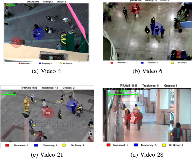
Fig. 8. Frames of videos 4, 6, 21 and 28. Red circles describe permanent groups while blue circles illustrate temporary groups. Yellow dots represent non-grouped people.
