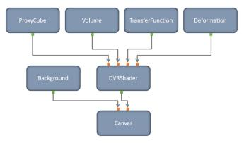
Fig. 9: Volrend's dataflow network. We chose this type of architecture because it provides more flexibility when creating and adding new components to the program.
