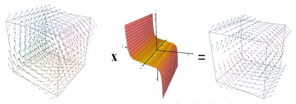
Fig. 7: A basic vector field representing a rotation around the x axis  $\vec{v}(x, y, z) = (0, -z, y)$  (left image) multiplied by the function  $h(z) = \arctan(10 * z)/(\pi/2)$  (middle image) creates the twist vector field (right image).
