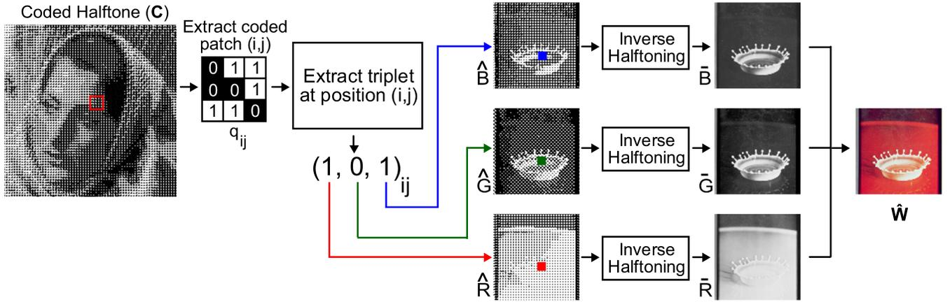
Fig. 2. Extraction of color watermark from encoded halftone.
