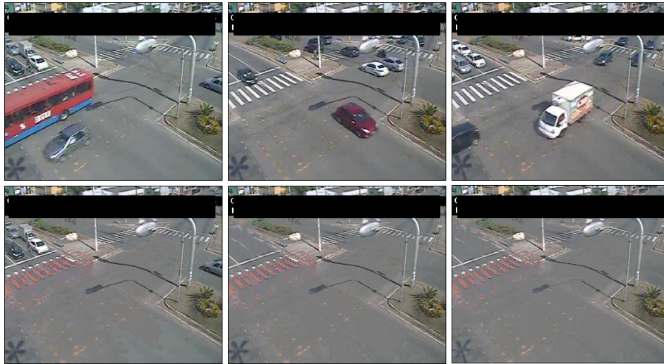
Fig. 1. Background modeling and the intersection problem: first row shows subsequent moments of a traffic video obtained from the monitoring of an intersection. Because the traffic light is switching between each opposite direction, there are always occlusion due to vehicles stopped in a red light. Second row shows the correspondent background models produced by the proposed method, CRON. The method is capable of learning the background whenever background pixels become visible, so that background consistency is preserved even when the vehicles stop again.
