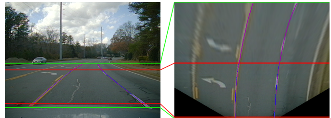
Fig. 8. Regions of interest: (a) red lines are the annotation boundaries and green lines are the boundaries of our region of interest. (b) The full IPM image is our region of interest. The blue dots represent the annotation that came with the dataset, and the purple dots represent our in-house annotation.
