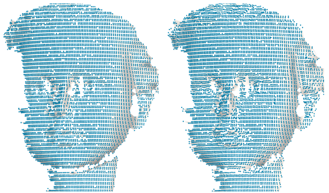
Fig. 9. Denoised a real scanned model with raw noise.
