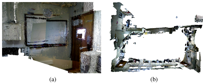
Fig. 11. Map errors from pairwise alignment by strategies (A) and (B), on subfigures (a) and (b), respectively. In this experiment, the key frame ids were provided by our methodology.
