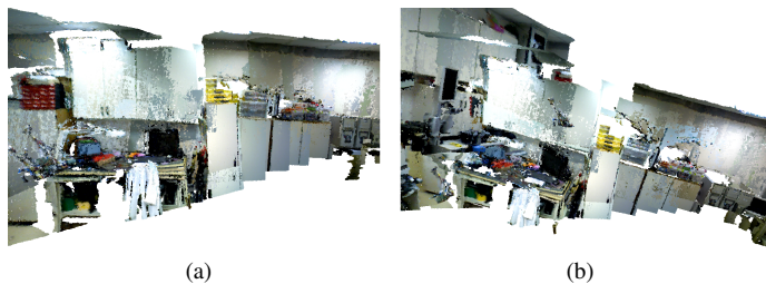
Fig. 10. Comparison of loop closing region as obtained from all strategies. A discontinuity can be spotted in the cabinet on the right, in (a); the same occurs in (b), with several other discontinuities that makes it the worst map estimated.
