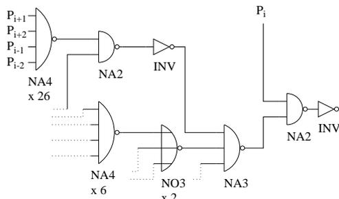
Figure 2: Schematic of a VLSI implementation for  $k = 2$
