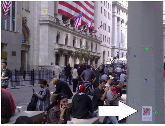
Fig. 16. FP=12 and QR code correctly detected.
