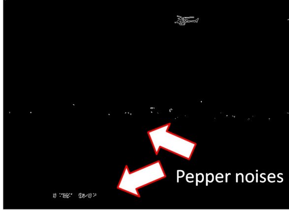
Figure 9. Residue image with Sobel method
