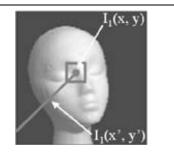
Figure 2. For computing  $I_2(x,y)$ , we sum the contributions  $G(x,x_0)I_1(x_0,y_0)$  from all those sites which precede (x,y) on the scan line of the required direction.
