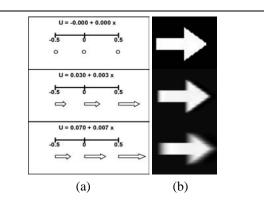
Figure 6. (a) Illustration of the behavior of U. (b) Translation simulation. From top to bottom: input image and *G*-filtered sequence for parameter values (u, u') = (0.03, 0.003), and (0.07, 0.007), with  $\theta = 0^{\circ}$ .
