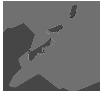
Figure 12. Detail of the Lake Superior. Approximated boundary of the small islands. Original boundaries are represented by line contours, and the final triangulated regions are filled.
