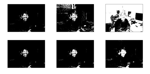
Figure 7: Thresholded images for the single-gaussian model (top row) and the double-gaussian model (bottom row). First collumn: segmented images at point (a); second collumn: segmented images at point (b); third collumn: segmented images at point (c) of fig. 6. It can be seen that, despite the fact that true positive rates are the same in each collumn, the double-gaussian model has lower false positive rates.
