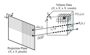
Figure 1: General scheme of a ray casting algorithm.
