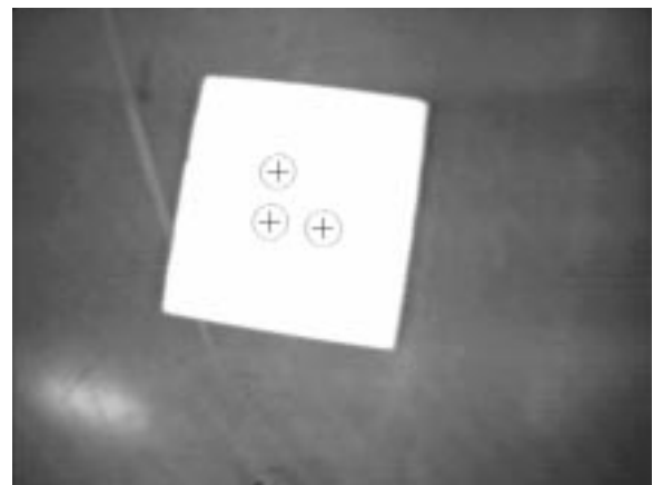
Figure 10: The markers of the artificial beacon as seen in the system graphic interface during tracking from the onboard camera.
