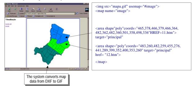
The system is able to convert the data from the specialized formats to generic formats that can be put on the Web. The map data is converted to a GIF file that is associated with a HTML file with the Map tag, which allows the image to be "clickable". When the user selects a polygon on the image, the browser will show another HTML document with information about the data related to that polygon.
