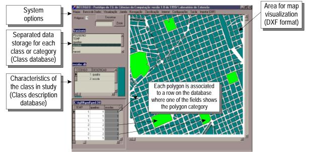
The image above shows an screen of **Intergeo** - an off-line system that is able to associate DXF vector-coordinate files with data bases, which can be used for geographical database search and visualization and for creation of files that allow the publishing of these maps on the Internet.
