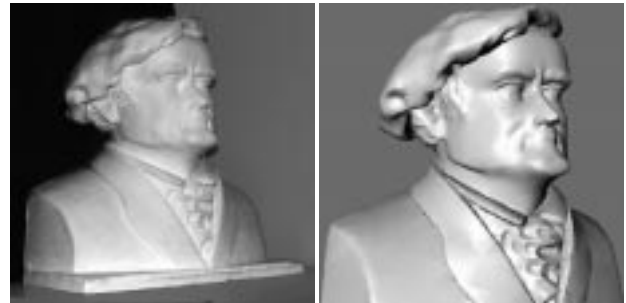
Figure 1: (a) plaster bust of composer Richard Wagner (b) 3D model reconstructed from 27 scanned range images
