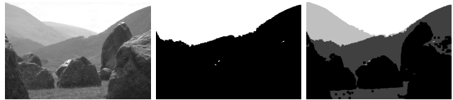
Fig. 2. (left image) a natural image; (middle image) the first segmentation with q = 0.46 achieving R_B and R_F ; (right image) the final segmentation with q = 0.15 and q = 0.73 for the previous R_A and R_F , respectively.
