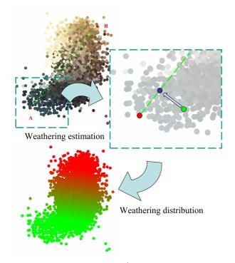
Figure 5. Consider the line segment  $\overrightarrow{AB}$ . The weathering degree of a point (green) in the appearance map corresponds to the position of the closest point (blue) in the segment.
