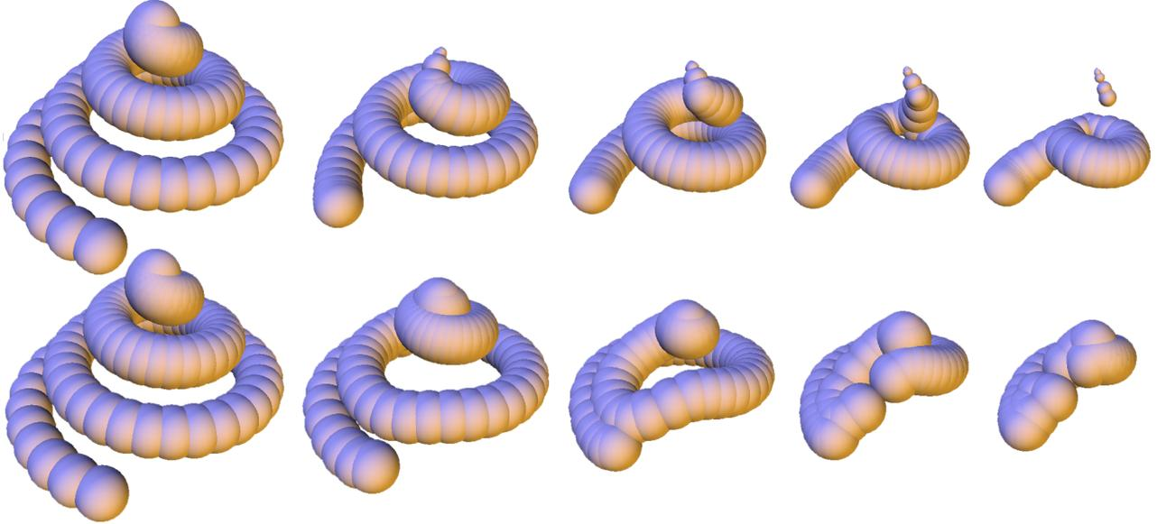
Figure 7. Gaussian filters in space (top) and along the medial axis (bottom) on the same example as Figure 4 fail in avoiding self-intersection.
