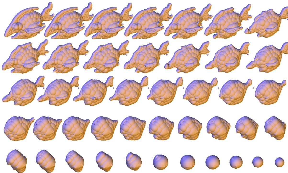
Figure 10. Some of the 300 iterations of our smoothing applied to an RBF model of a fish, on the positive poles: similarly to curvature motions, our smoothing convexifies the shape in finite time.
