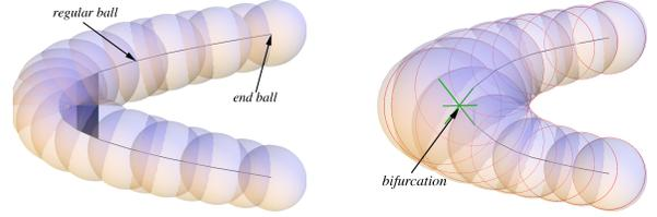
Figure 3. The 2D curvature motion for union of disk deforms bifurcation balls as means of regular motions (green lines).
