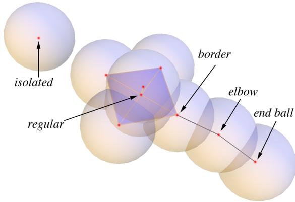
Figure 5. Classification of the balls according to their adjacency in the medial axis.
