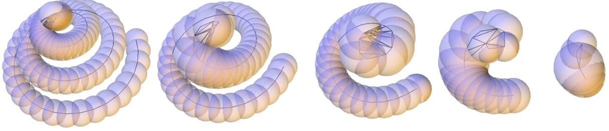
Figure 4. Our scale-space smoothing on a spirally shaped, after 1, 20, 40, 60 and 80 iterations: the movement avoids self-intersection, even in delicate cases. The lines show the medial axis edges along the deformation.
