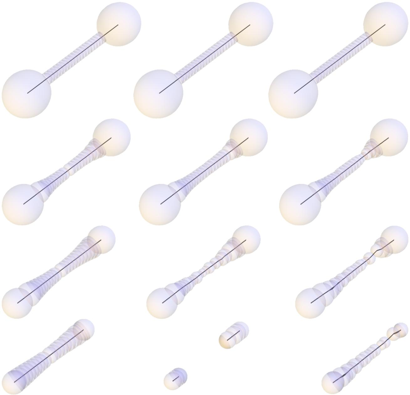
Figure 11. Smoothing a dumbbell shape from min curvature-like motion (left) and mean curvature-like motion (center) and max curvature-like motion (right), after 50, 100, 150 and 200 iterations.
