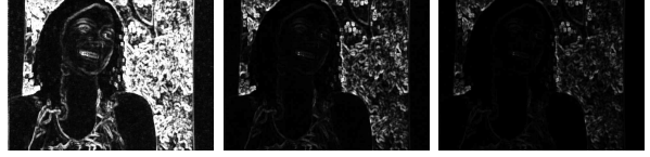
Figure 6. Image of boundary probabilities taking the maximum value of a 8-connected neighborhood. Darker pixels have smaller probabilities (left) \sigma_C = 5 (center) \sigma_C = 15 (right) \sigma_C = 25 .
