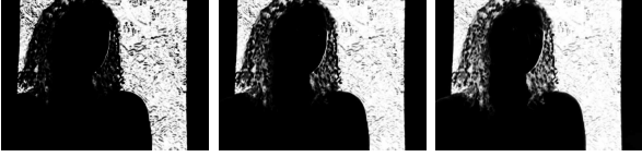
Figure 4. Images of background probabilities. Darker pixels have smaller probabilities (left) \sigma_L = 15 (center) \sigma_L = 25 (right) \sigma_L = 35 .
