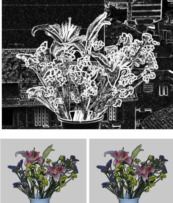
Figure 10. (upper)Boundary probabilities with \sigma_C = 5 . The resultant segmentation using different parameters: (lower-left) \sigma_L = 25 , \sigma_C = 10 , (lower-right) \sigma_L = 15 , \sigma_C = 5 .
