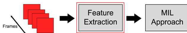
Fig. 1. The SSOC approach proposed in this paper focuses on the feature extraction step (represented by the red rectangle) in the video surveillance anomaly detection pipeline. To obtain the results, existing MIL methods are employed.
