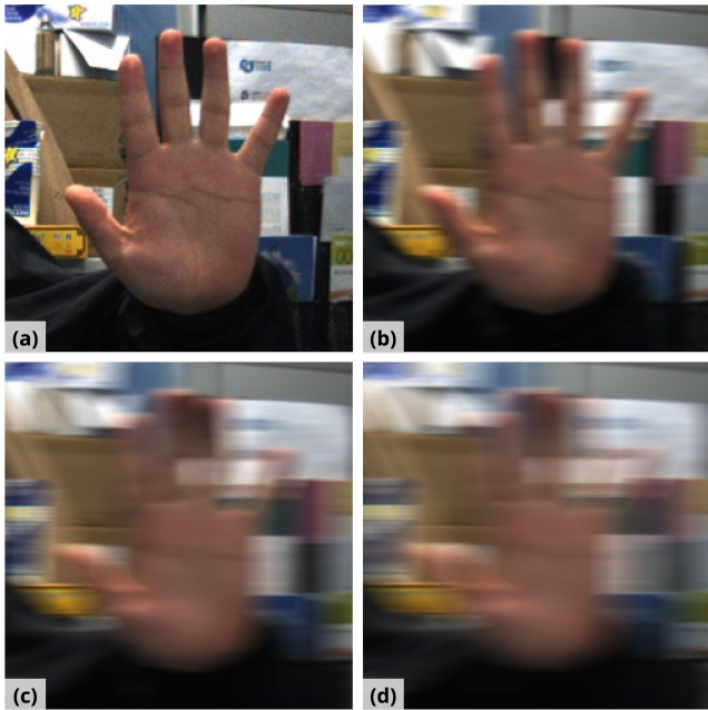
Fig. 2. An image from the S-val set that was selected and processed using horizontal motion blur. (a) Original image, without processing. (b) Original image blurred with horizontal motion blur with kernel size of 15 \times 15 , (c) 30 \times 30 and (d) 45 \times 45 .
