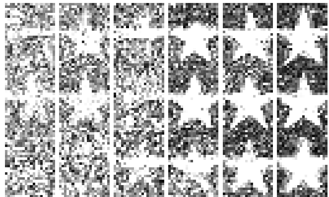
Fig. 15: Integrated LIA reconstructions of a star at different frame duration by three users. The top row is from User A. The middle row is from User B. The last row is from User C. Stimulus frame duration are increasing from left to right: 0.25 s, 0.5 s, 0.75 s, 1.0 s, 2.0 s and 4.0 s.
